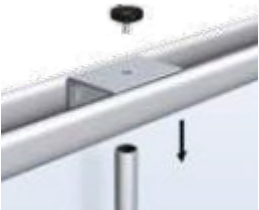
Double frames attach easily to upright. View from both sides.
